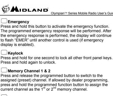
assigned (preset) channel. If allowed by dealer programming, press and hold the programmed function button to assign the current channel as the 1<sup>st</sup> or 2<sup>nd</sup> memory channel.
